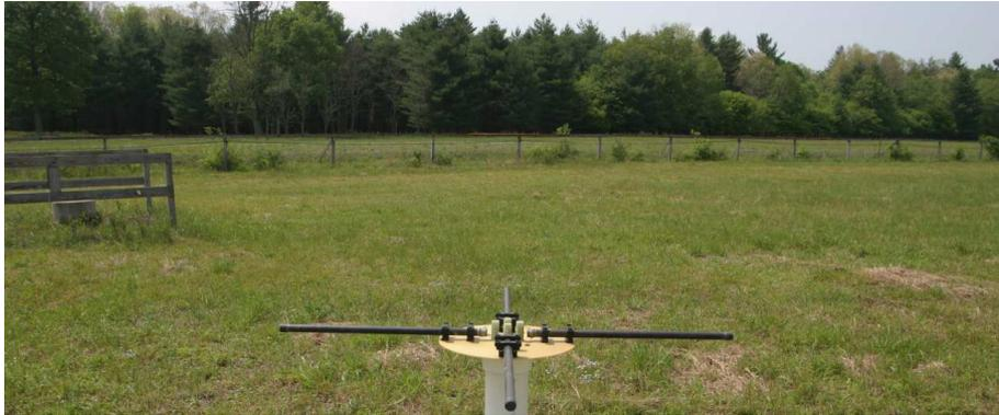
Figure 4.4: A long cable housing believed to be responsible for the observed horizontal fringes
