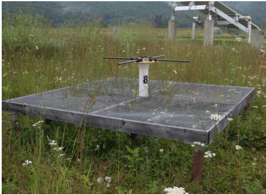
Figure 4.5: Antenna and groundscreen. Please note the warp in the nearest quadrant of the groundscreen
