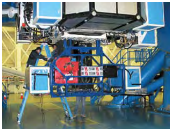
Figure 2. NICI installed on the Gemini South telescope, getting ready for its first commissioning night on the sky.
