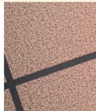
Chromium microdot apodizer with astrometric grid
