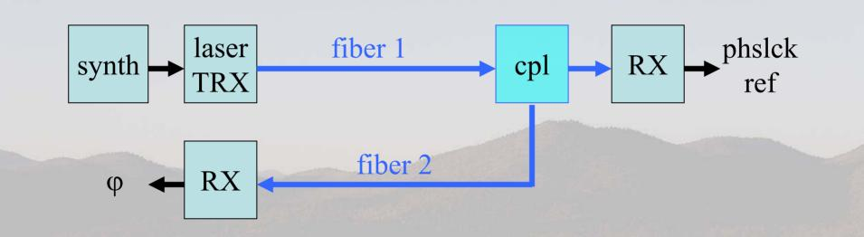
• no electronics at the antenna, just a fiber coupler
