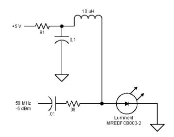
**Test results** (50 MHz rcvr #1, tested 10/15/04; absorber pasted inside lid): With -20 dBm optical power into receiver (photocurrent monitor = 0.25 V, LED is green), the signal to noise ratio of the 50 MHz tone is roughly 500, which corresponds to an rms phase error of 0.03 radians.
