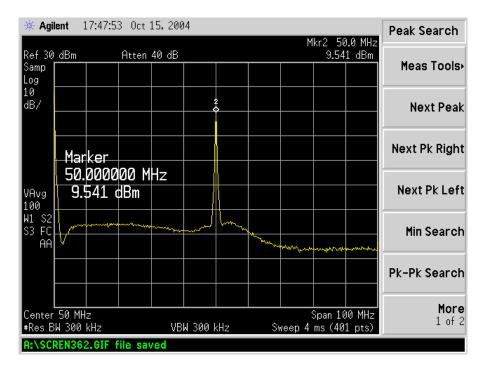
**Harmonics:** At the highest likely optical power level (-15 dBm; photodiode current monitor = 0.8 V), the 2<sup>nd</sup> and 3<sup>rd</sup> harmonics are still more than 50 dB below the peak:
