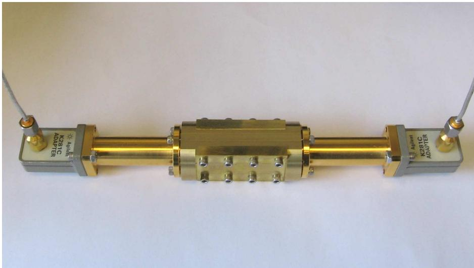
Fig. 7.— Photo of K-band scale model (a) under test.
