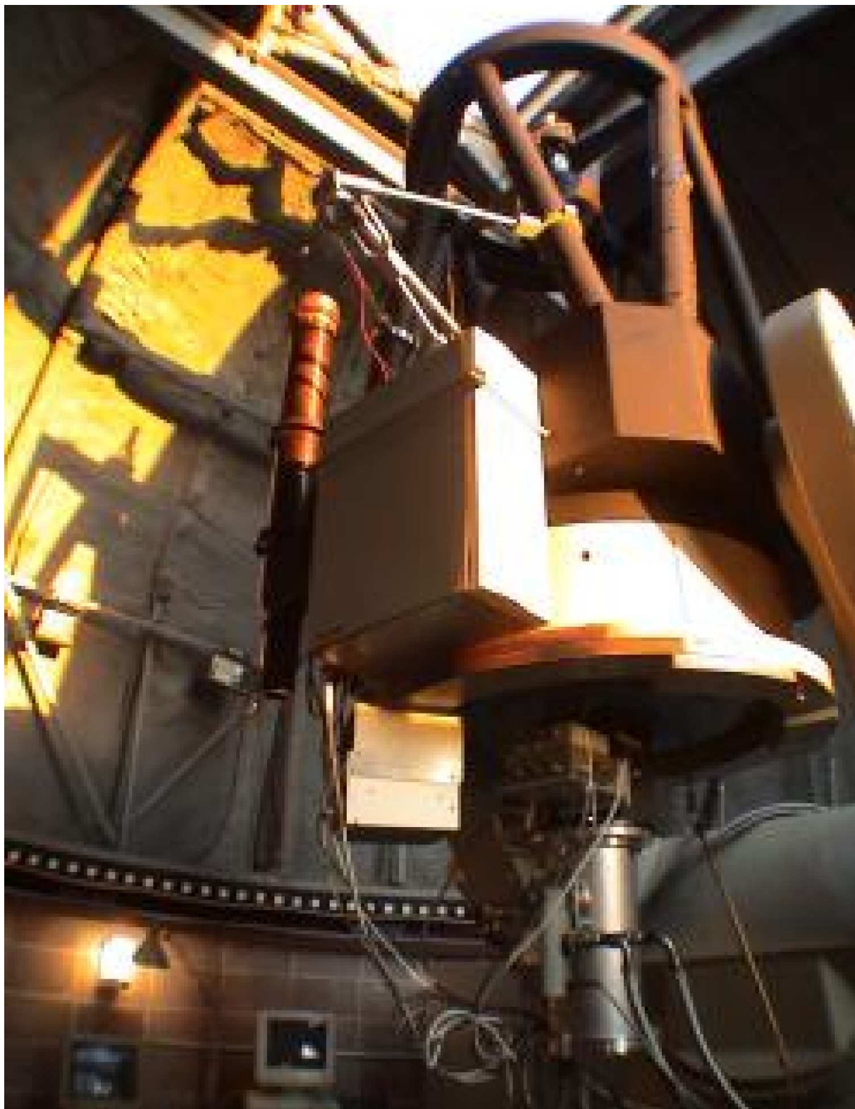
Fig. 6.— The robotic 30-inch reflector at Leuschner Observatory (Lafayette, CA). An infrared camera is installed at the Cassegrain focus.
