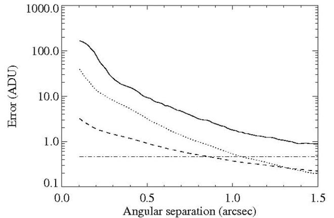
FIG. 19.—Real error (solid line) compared to estimates of the photon noise (dashed line), read noise (dash-dotted line), and flat-field noise (dotted line) for epoch 3. The real noise is dominated by the residual speckle noise. The innermost region (within about  $0.1''$ ) is saturated and does not provide any meaningful information about the real error.
