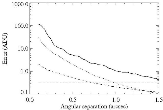
FIG. 18.—Real error (solid line) compared to estimates of the photon noise (dashed line), read noise (dash-dotted line), and flat-field noise (dotted line) for epoch 2. The real noise is dominated by the residual speckle noise, except in the very outermost part where the read noise seems to be significant. The innermost region (within about  $0.1''$ ) is saturated and does not provide any meaningful information about the real error.
