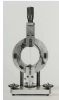
◆ Phase contrast mask with phase shifter.
