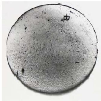
◆ Phase contrast image of small defects of a lens.
