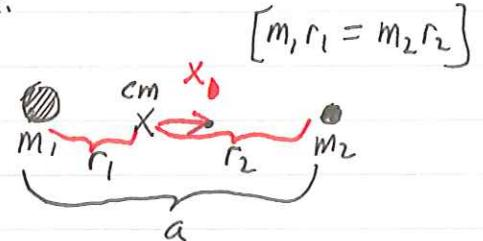
$$0 = \frac{-GM_1}{(r_1+x)^2} + \frac{GM_2}{(r_2-x)^2} + \frac{G(m_1+m_2)x}{a^3}, \text{ where } a \equiv r_1+r_2$$
