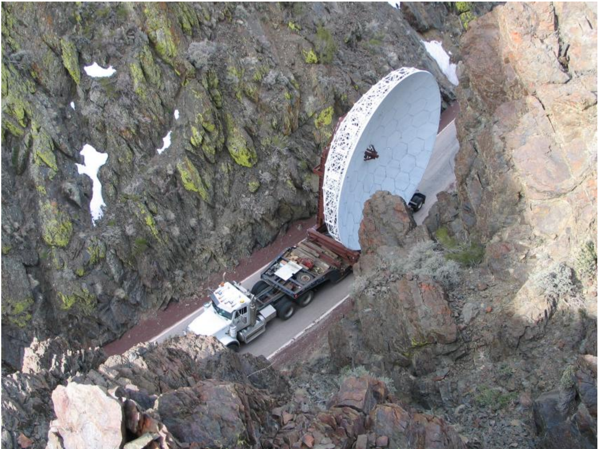
Figure 15: Moving 10m antennas 38 thro the narrows to CARMA
