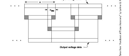
$DM = 71, f = 1.4 \, GHz$ ,  $\Delta f = 100 \, Mhz \rightarrow fft_{len} > 4.2 \, Mpts!!$  $DM = 71, f = 900 \, MHz$ ,  $\Delta f = 100 \, Mhz \rightarrow fft_{len} > 16 \, Mpts!!!!$
