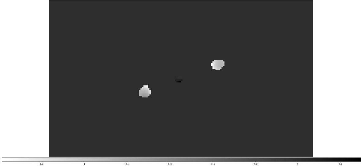
Fig. 24.— Spectral index, \alpha , across the radio lobes by comparing CARMA map at 100 GHz and VLA map at 15GHz convolved to a lower resolution. \alpha becomes more negative (spectrum steepens) further from the hotspots, suggesting evolution of the radiation.
